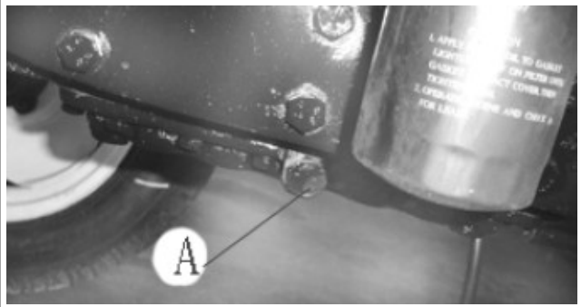
Figure 5-15 Replacement of Oil in Engine Oil Pan
