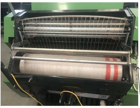
By adjusting the spring in different holes, adjust the tension of the pressure bar; make it press the net always.
